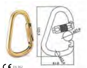
LX07 Carabiner / Twist Lock Alloy Steel MBL: 35kn
